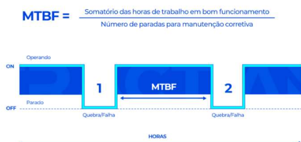
Figura 4 – Fórmula MTBF: Mean Time Between Failures
