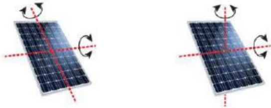
Figure 3 – Tip Tilt and Azimuth-Altitude Trackers and their axes of rotation.
