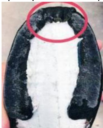
Figure 3. Defective sole. Figure 4. Cutting on the skin
