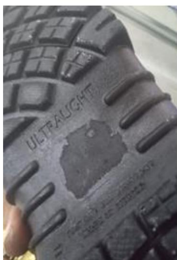
Figure 3. Defective sole. Figure 4. Cutting on the skin
