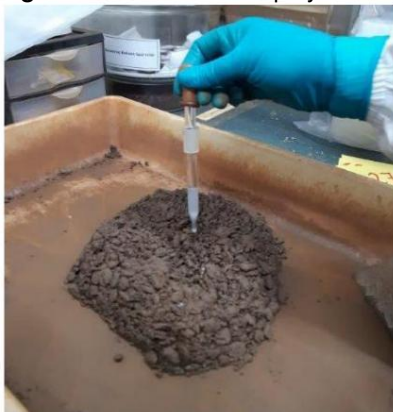
Figure 1: Addition of the polymer to the iron ore sample.
